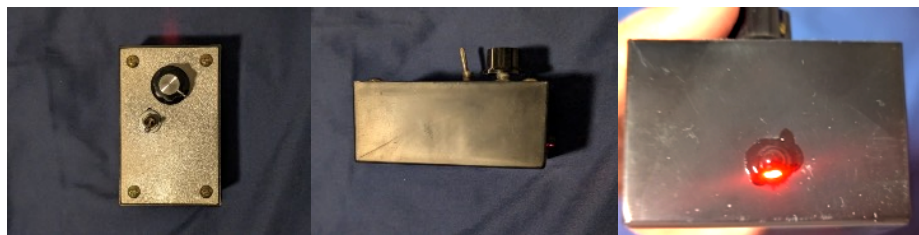
Top, side, and front views of the Fiscus light. Dimensions: 82 mm X 52 mm X 36 mm; Weight: ~100 grams. Photos by Alex Samuel.
